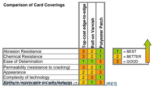
It is important to keep intended usage considerations in mind when making decisions about added security and personalisation features of card design. For example, the smart card industry recommends applying a protective coating or laminates to virtually every smart card containing color photos and also suggests that all forms of personalisation should be kept away from card edges and other wear-prone areas. Other personalization and security
